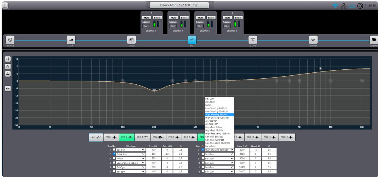
From the Home page tap the PEQ tab to access the EQ main page. From this page you can dial in numeric values for the 12 EQ filters.. Each EQ can be set to a choice of 16 filter types: Bell-Sym, Bell-Asym, Notch, Low-Shelf 6dB or 12dB, High-Shelf 6dB or 12dB, All-Pass 90° or 180°, High-Pass 6dB or 12dB, High-Pass Vari-Q 12dB, Low-Pass 6dB or 12dB, Low-Pass Vari-Q 12dB, Band-Pass.
