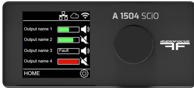
The front panel gives the user access to the status of the amplifier and also gives the user the ability to set IP parameters and basic audio settings.
