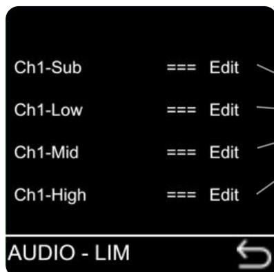
From the Limiter sub menu, you can select with the encoder an amplifier channels limiter page to edit.
