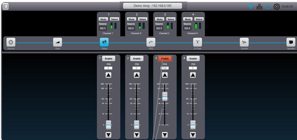
Delay: opens a window where you can set the delay in ms of the four channels, regardless of what channel is selected. Values can be set with the fader, keyboard arrows or by dialling in the desired level. Delays can be toggled between enable and disable for A-B comparison.
