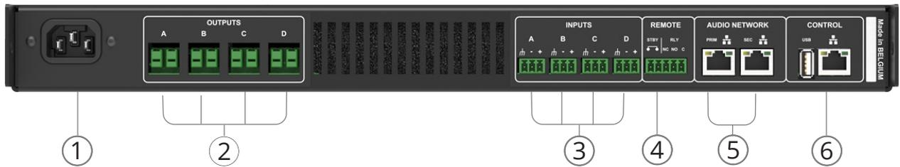
1. IEC connector accepts worldwide operation from 100-240Vac. A Series must be grounded (earthed) with the safety ground pin to the mains distribution system. NEVER disconnect the earth (ground) pin on the mains cable (AC power cord).
