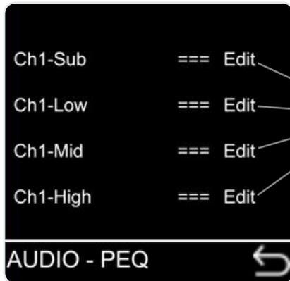
From the Parametric Equalizer sub menu, you can select with the encoder an amplifier channels Eq page to edit.
