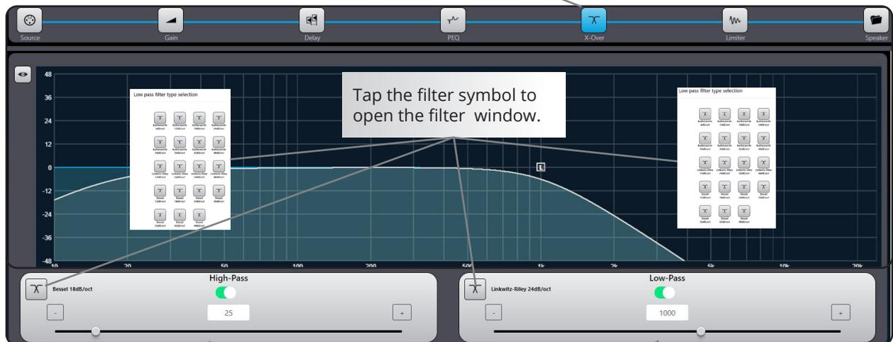
Adjusting the Filter parameters can be done in multiple ways: use the sliders and tap the +/- buttons for fine adjustments or use the on screen drag function with mouse, pen or finger gestures. Both filters can be set from 10 Hz to 22 kHz
