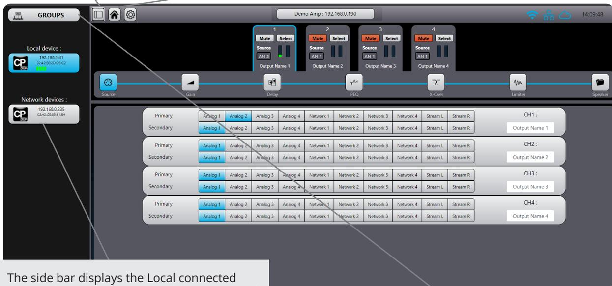
The side bar displays the Local connected device (if any) together with all the connected devices found on the network.
