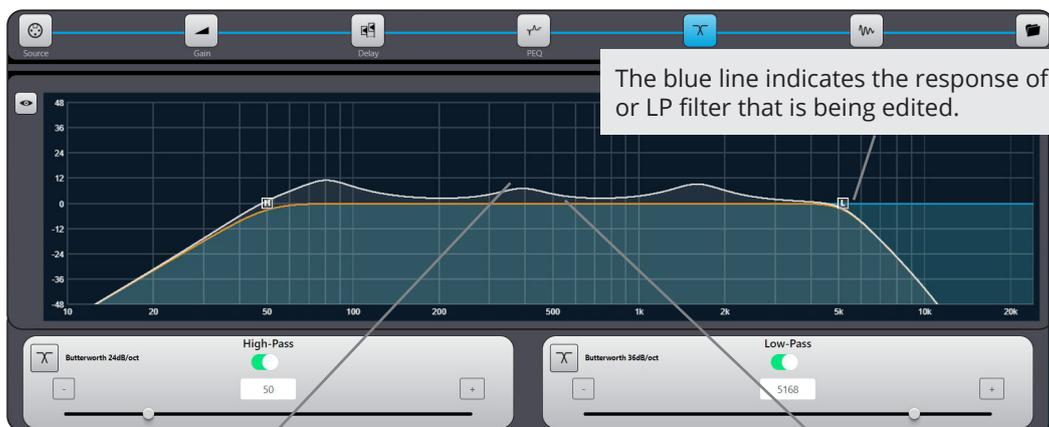
The white line reproduces the total response of the amplifier channel including all PEQ, High and Low-Pass filter.
