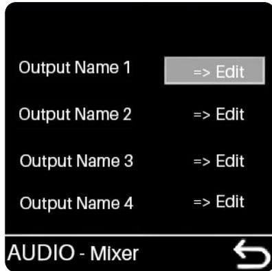
From the mixer sub menu, you can select the combination of inputs for each amplifier channel. There are twelve input options for each channel. Analog 1- 4, Stream L, Stream R, freq gen, pink noise and Network 1 - 4. The digital option card options are DANTE or AVB.
